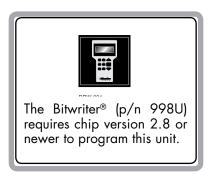
Bitwriters with a date code of 6a or older require an IC upgrade (p/n 998M). Some bitwriters with a date code of 6B do not require the IC upgrade, refer to tech tip # 1112 for more information.
