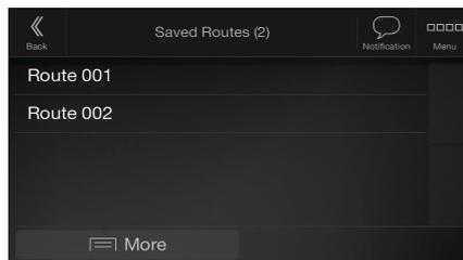
By selecting a previously saved route, Alpine Navigation System recalculates the route using the saved destination and/or the waypoints.
