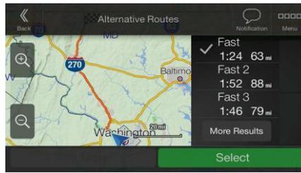
If there are suitable alternatives calculated with the route planning method that is selected in Route preferences (page 72), they are shown on top of the list. Routes with other route planning methods are shown at the bottom of the list.
