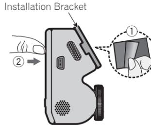
Use extreme care as the double-sided tape on the Installation Bracket in (①) is extremely strong, and it will be difficult to reapply the tape once it has been applied.
