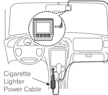
The power terminal will be extremely hot immediately after using the cigarette lighter. The tip of the Cigarette Lighter Power Cable may melt or short circuit if it is plugged in while hot. Wait for the terminal to cool before plugging in the Cigarette Lighter Power Cable.
