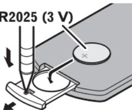
Insert the CR2025 (3 V) battery with the plus (+) and minus (-) poles orientated properly.
