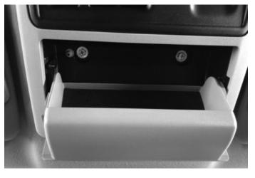
10 Remove the plastic fastener on the driver's kick panel by turning left. Unsnap and remove the kick panel.
