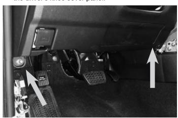
8 Extract (2) 10mm screws from the eyewear compartment and pull down to release it.
