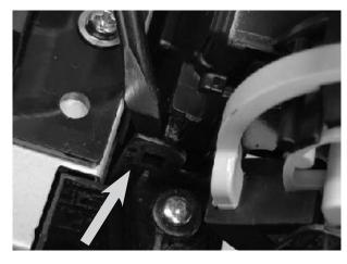
4 Use a small flat head screw driver to release the lock tab on the hazard light connector at the radio chassis.
