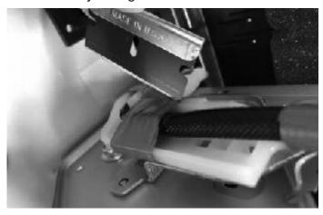
2 Use a small flat head screw driver to release the lock tabs on the outer side of the vent.
