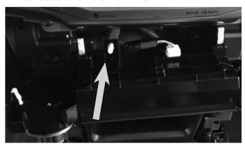
5 Use a panel removal tool to release the clips and remove the factory radio.
