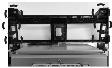
8 Remove the top and vent trims. Note: be sure to retain all screws as they will be used on the new radio panel.
