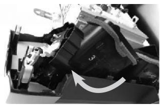
5 Use a razor blade to cut the tape securing the hazard light switch harness and remove it. NOTE: Cut away from the harness so the wiring is not accidentally damaged.
