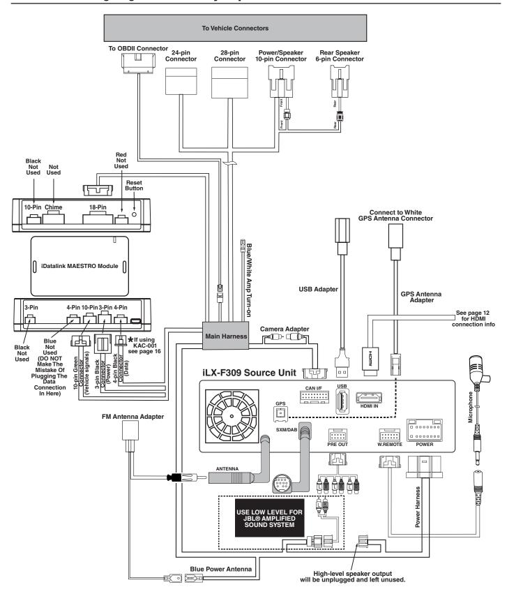
There is no way to integrate the factory SiriusXM tuner. Once the radio is removed, the factory SiriusXM is removed. As the title states, SiriusXM requires a tuner sold separately. This diagram shows how to integrate the antenna connection.
