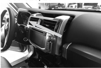
2 Use a panel removal tool to release the HVAC control panel.
