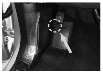
12 Use a panel removal tool to release the clips and remove the driver's knee cover panel.
