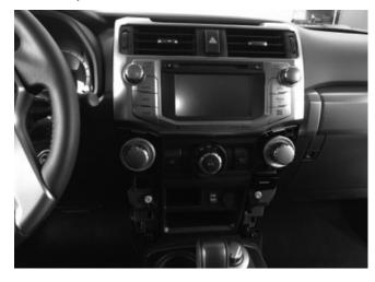
4 Use a 10mm socket to extract the (4) screws below the factory radio.
