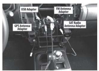
8 Mount the iLX-F309FRN using the factory screws. Note: Kit only requires (2) 10mm screws. Place the additional (2) 10mm screws back into the factory location in case they are needed in the future.
