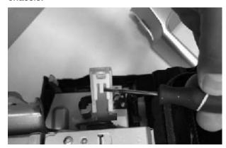
6 Disconnect the hazard light switch and remove it by pushing it from the rear to the front of the radio panel.
