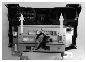
3 Tilt, lift, and remove both vents.
