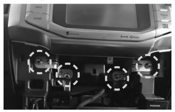
**6** Use a panel removal tool to remove the "SRS Curtain Airbag" screw cover.
