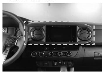
2 Use a 10mm socket to extract (4) 10mm screws from the factory radio, disconnect and remove it.
