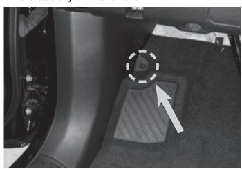
8 Extract (3) 10mm screws from the driver's side knee cover, release the clips and remove it.
