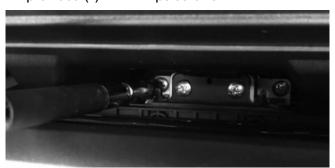
11 Slide screw cover into place. Note: Failure to mount the cover properly may cause the iLX-F309TCM to not turn ON or function properly.
