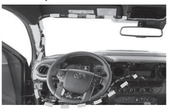
5 Connect the radio harness (according to the vehicles sound system) following the system diagram on pages 9 or 10.
