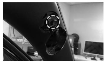
5 Use a panel removal tool to release the clips on the eye wear storage compartment and remove it.
