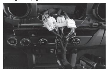
4 Connect the FM, GPS, SAT Radio Antenna and USB adapters.
