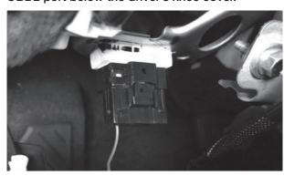
3 Route the microphone down to the OBD2 connector and route both Microphone and OBD2 cables to the radio cavity as shown below.
