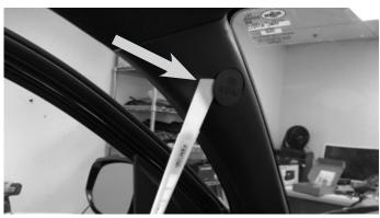
4 Use a 10mm socket to extract the screw from the A pillar panel cover.
