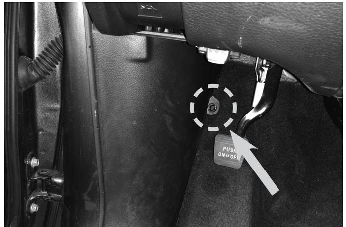
**9** Use a 10mm socket to extract (2) 10mm screws from the driver's side knee cover panel.
