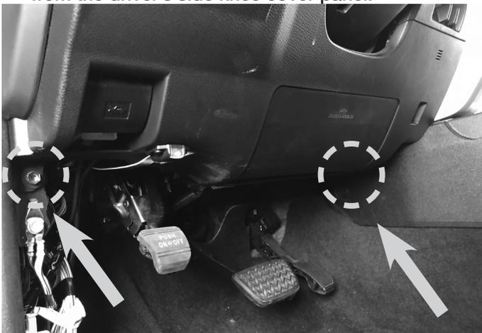
**10** Use a panel removal tool to release the clips on the knee cover panel and remove it.
