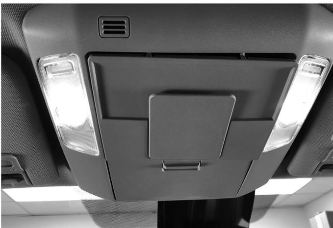
**12** Open the eyewear compartment to reveal (2) T20 Torx screws. Extract (4) Torx screws from the entire assembly and remove it.
