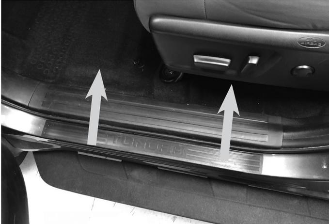
**8** Remove the plastic nut on the driver's kick panel and carefully lift the kick panel to remove it.
