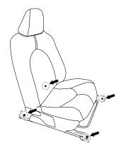
8 Tilt the passenger seat towards the back to reveal (4) connectors. Disconnect and remove the seat.
