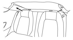
2 Disconnect the ANC microphone and replace all removed components to their corresponding location.
