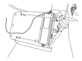
12 Route the main harness to the radio location and secure any excess wiring with the provided cable ties.
