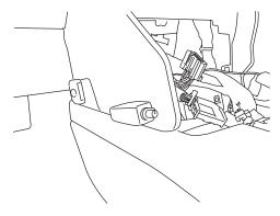
8 Use a 10mm socket to mount the firewall bracket to the factory stud below the fan assembly. Note: Additional adjustment may be required (right to left) to mount the amplifier assembly.
