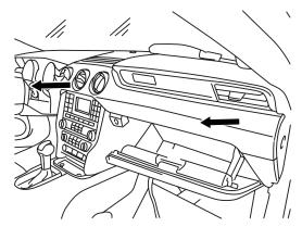
3 Use a panel removal tool to release and remove the plastic tray. Note: 2015 - 2017 models only. 2018 -Up skip to next step.
