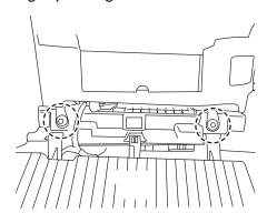
6 In some cases the clips may need to be opened slightly to allow sliding into place.
