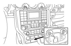
6 Extract (4) 7mm screws and remove the radio.
