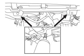
4 Release the globe box compartment by pressing the side tabs towards each other and releasing the shock on the right side.
