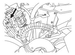
2 Route the power cable thru the rubber grommet on the firewall on the passenger side foot well.
