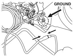
10 Roll and secure the excess cabling using the provided cable ties.
