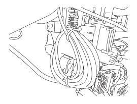
11 Connect the main harness and subwoofer level remote to the amplifier assembly.
