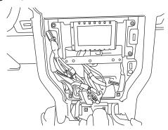
14 Mount the amplifier assembly using the provide 8-32" Phillips screws.
