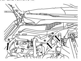
2 Use a 10mm socket to loosen the Negative (-) battery terminal and disconnect it.
