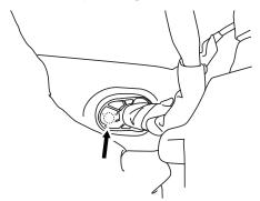
3 Locate (2) hole openings below the globe box and enlarge them to 1/2"using a step drill.
