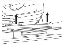
2 Remove the passenger side kick panel by carefully lifting up.
