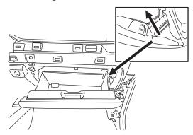
5 Remove (2) 8mm screws from the lower glove box compartment cavity and attach the (2) hook mounting clips using the same screws.
