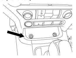
2 Remove the rubber cover from the tray in front of the shifter to reveal (2) 7mm screws and extract them.
