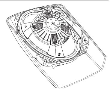
NOTE: It is easiest to place the grill into the hole that has been cut into the lid and place upside down on a bench. Then place the appropriate mounting ring onto the grille, along with the speaker. Secure with the supplied screws.
