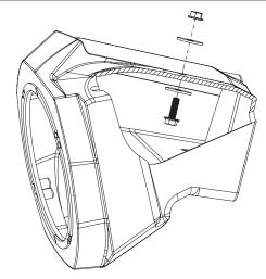
Step 3. Secure the enclosure using supplied hardware.
