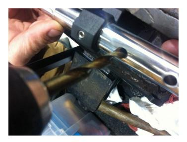
6) Clean sharp edges from newly drilled hole
