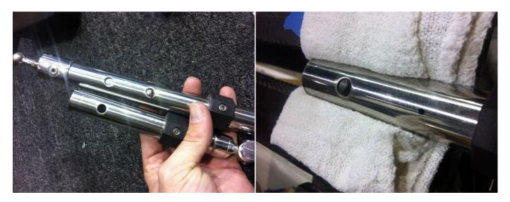
5) Use a punch and tap a starter point for the drill bit. Drill new hole with a 9/32 drill bit.
