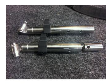
2) Disassemble the arm and place the pole in vice and cut with pipe cutter just below first hole (1 7/8")
