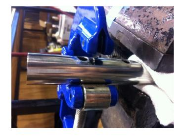
3) Clean out sharp burs and edges from the cutting process so inner pole will slide without scaring
