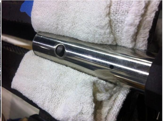
5) Use a punch and tap a starter point for the drill bit. Drill new hole with a 9/32 drill bit.
