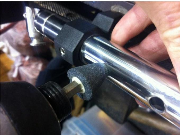
7) File out inside to remove sharp metal debris from inside pole
