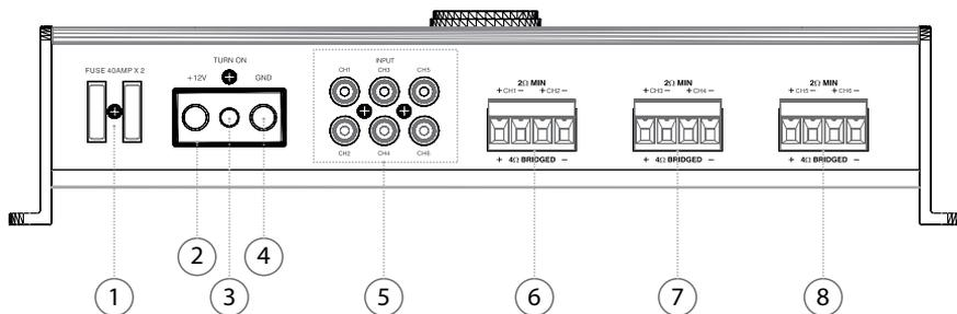
1. **Fuses** – The fuses protect the amplifier against internal electrical damage and are meant to protect the amplifier only. All other power connections should be fused at the source
