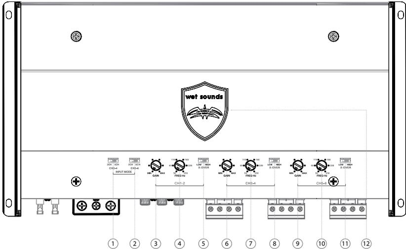
1. **Channel 3-4 Input Switch** – Adjusting this switch to 2 channel input and connecting only the CH 1/2 inputs allows the amplifier to have 4 channel output.
