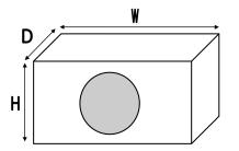
Sealed Dimensions: Height (H) : 10" (254 mm) Depth (D) : 8" (203 mm) Width (W) : 10" (254 mm) Cutout Diameter: 7-1/4" (184 mm)
