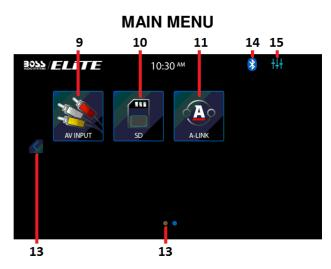
At **MAIN MENU**, touch the icon of the desired mode on screen and the unit will then enter into the mode that selected for operation.
