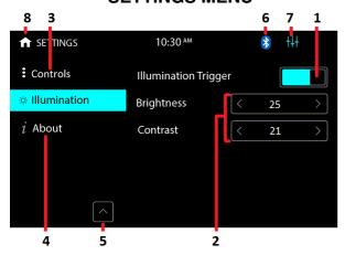
1. Touch to turn on or off of headlamp detection of the car.
