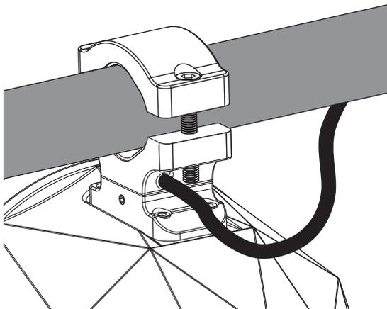
Step 9: Slide the wire jacket down thru the hole with grommet and wire. Snake the wire down to the bottom of the tower tube in a location that the wires can be attached to the audio (and lighting) system. Solder or butt connect the speaker wire coming from the tower to the speaker wire to the system. Then heat-shrink it for added protection from water/moisture.
