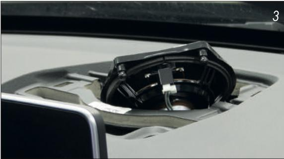
*Remove existing plugs from the loudspeaker.*
