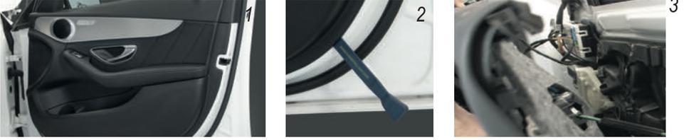
Remove the two screws on the door handle (TX27) and start to remove the clamps on the door panel from the bottom and then pull it out. Now remove all the plugs that are connected to the door trim
