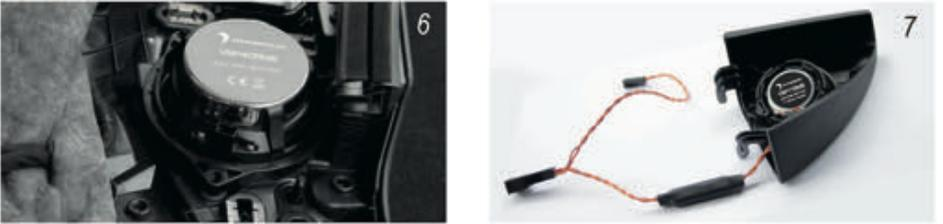
Now mount the Diamond Audio speaker in the slot by pushing it in. Then remove the old tweeter from the mirror triangle, if available. Afterwards attach the Musway tweeter.
