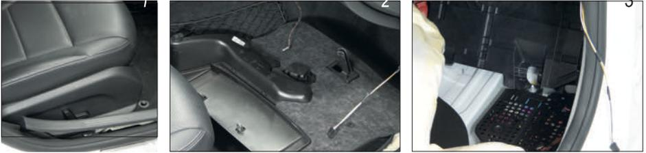
Remove the door strip and the cover under the glove. If present, remove the plug from the cover.
