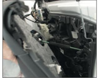
Remove the two screws on the door handle (TX27) and carefully lever the door trim out (from bottom to top). Now remove all the plugs that are connected to the door trim.
