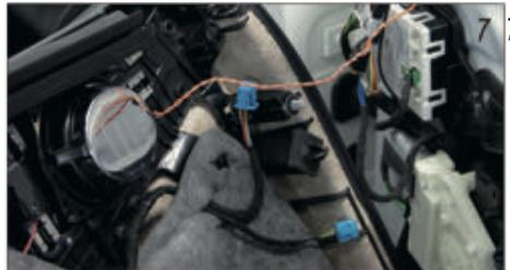
Now mount the Diamond Audio speaker by pushing it in and connect it to the factory cable of your vehicle. Mount the door trim in reverse order.
