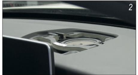
*Lever out the speaker grille. Then loosen the old speaker (lever out, not screwed).*
