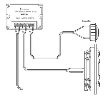
Each H65HS component crossover has a third set of outputs marked "RAF". This stands for Rear Acoustic Fill. This output can be used to power and additional speaker off the same channel without effecting the impedance load on the source unit. The level of this output is pre-determined at -10dB of attenuation, for a REAL "rear fill" This creates a much more real stereo image and a bigger sound stage
