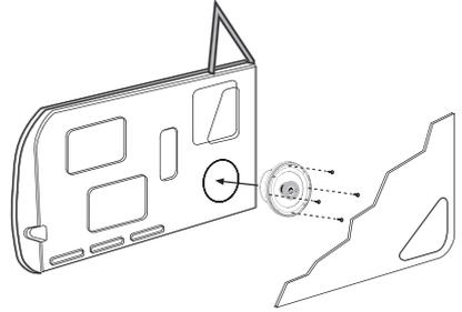
If you are mounting the speakers in the rear of the vehicle, there are often two options for achieving a good mount. Some speakers mount from the top side (from the interior) while other applications have the speakers mounted from the bottom side (from the trunk). In either case, a flat mounting surface and a good seal are still extremely important.
