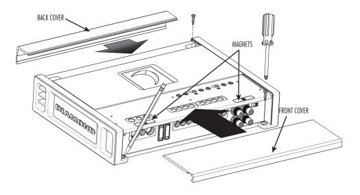
NOTE: These covers are both a friction fit as well as magnetic. There is a small "lip" on the front cover that clamps the front cover on tightly. Sometimes it can be somewhat hard to remove. Be careful, but forceful.
