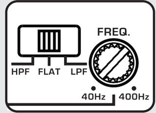
Placing the switch in the HPF position sets the amplifier to the High Pass Filter mode, enabling frequencies above the cutoff point to pass. Placing the switch in the LP position sets the amplifier to the Low Pass Filter mode, enabling frequencies below the cutoff point to pass. For system tuning begin with the frequency set at approximately 80Hz and fine tune up or down based on music choice and input level.
