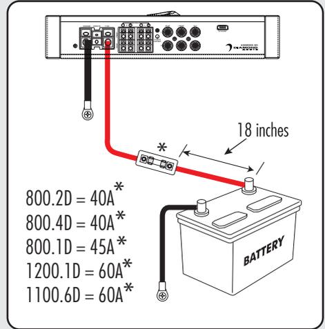
7. Securely mount the amplifier to the vehicle or amp rack. Be careful not to mount the amplifier on cardboard or plastic panels. Doing so may enable the screws to pull out from the panel due to road vibration or sudden vehicle stops.
