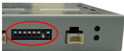
**\*Note: after adjusting Dip Switches, you must disconnect and reconnect power to the interface or the change will not be implemented.**
