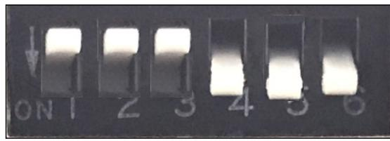
**FOR FRONT CAMERA ENSURE "DIP SWITCH 1" IS IN THE DOWN POSITION**
