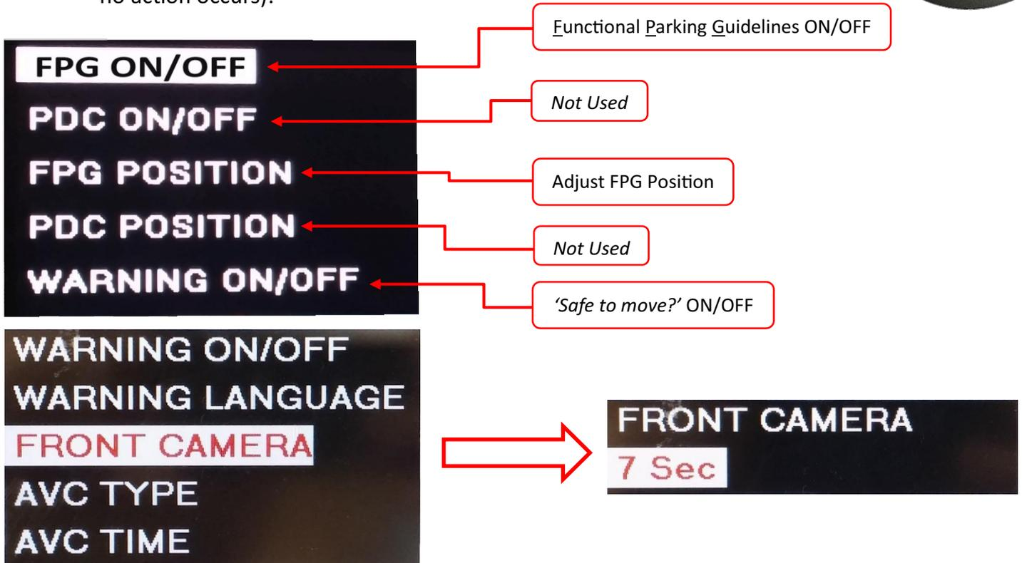
To activate **Front Camera timer**, scroll down using the remote arrow keys when in the menu to **FRONT CAMERA**. Once in this setting, press OK and choose (up/down) between 5, 7, 9 or 11 seconds for **auto-front switching timeout** (once the vehicle leaves reverse gear, the front camera input will stay active for pre-defined amount of time).
