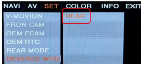
REAR shows the 'CAMERA' RCA (with no lines) when the green reverse wire is triggered.
