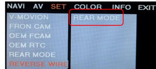
REAR MODE shows the 'CAMERA' RCA (with dynamic lines) when the green reverse wire is triggered.
