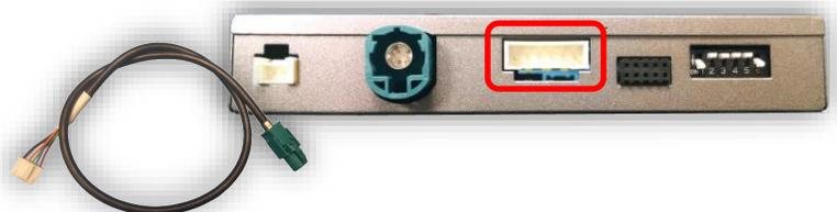
5. Connect the free end of the provided **LVDS Video Cable** (green) back to the factory radio at the bright **GREEN** cluster LCD port.
