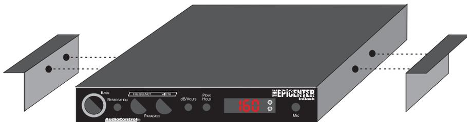
We have provided brackets to assist you in mounting The Epicenter InDash chassis under your dashboard or wherever you may choose. The screw holes on The Epicenter InDash chassis also allow for easy installation underneath a radio or with a dash kit. It is of utmost importance to mount The Epicenter InDash securely to avoid any undue stress or breakage from over acceleration or braking.
