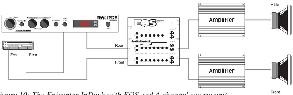
Figure 10: The Epicenter InDash with EQS and 4-channel source unit
