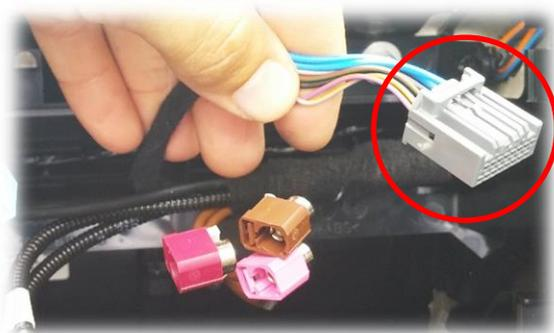
2. Connect the provided **SMB-RCA Adapter** to the screen at the port (typically purple) closest to the M.O.S.T Fiber Optic connector.
