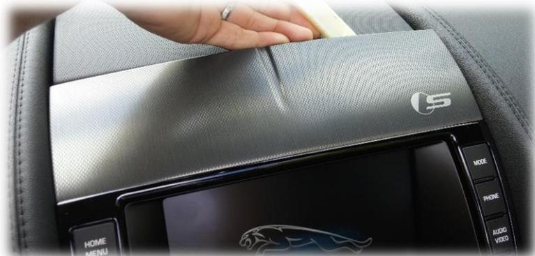
5. Remove (2x) Torx t20 screws securing the screen bezel:
