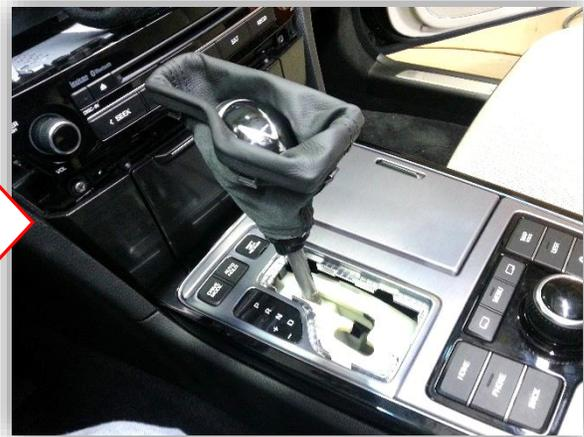
2. With a plastic panel tool, pry up and remove the lower console panel that houses the radio control knob. Disconnect all harnesses and carefully pass the shifter knob through the wider portion of where the boot was seated:
