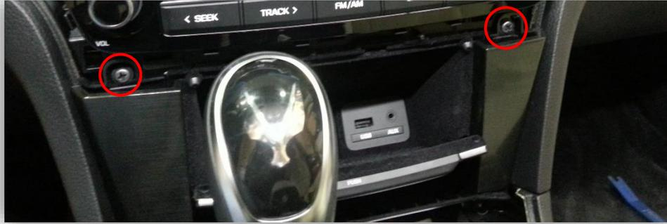
8. The lower dash pocket will be free now, pull straight out and up towards to, remove 3 connectors.
