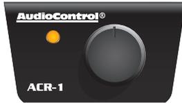
The optional AudioControl ACR-1 dash control is a remote level control for your LC-1.800 amplifier. It may be mounted under the dash using its own enclosure, or through a custom hole in the dash. The level control knob should be within reach of the driver, and in a spot where the LED is plainly visible. Disconnect the vehicle battery +12V and Ground connections before installation.
