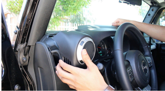
7. Raise the upper dash panel to release the radio bezel.
