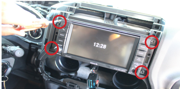
9. Remove the 4 screws holding the radio.
