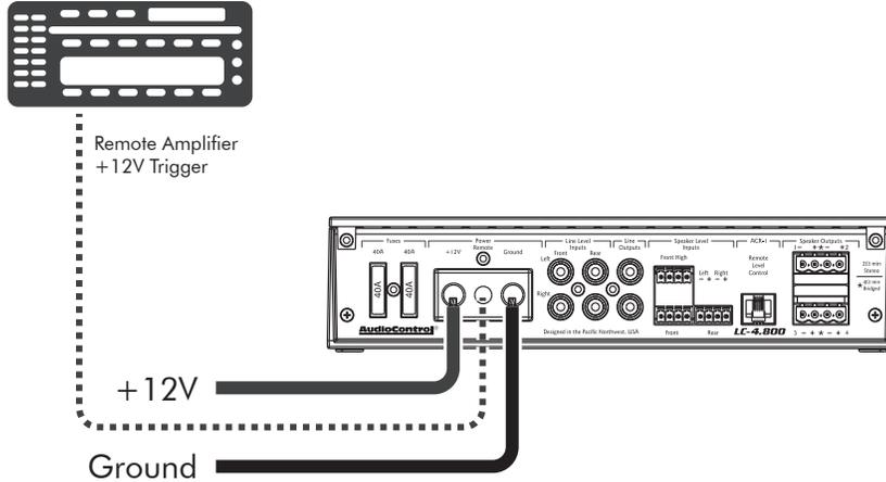
In this example, the head unit has a +12V trigger output that is connected to the LC-4.800's remote input terminal. When the head unit is turned on, it will turn on the LC-4.800 amplifier.
