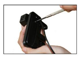
2. Remove the 4 screws holding the CMB-15T camera.
