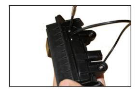
6. Put the camera back to the CMB-15T base and secure using the 4 screws.
