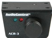
1. When the left (**BLUE**) LED is on, turn the remote knob clockwise to turn the level up, and counterclockwise to turn it down.
