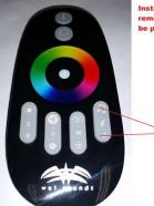
Instructions for pairing remote to rgbmcv2 if remote is not working. Only one remote can be paired to the controller.
