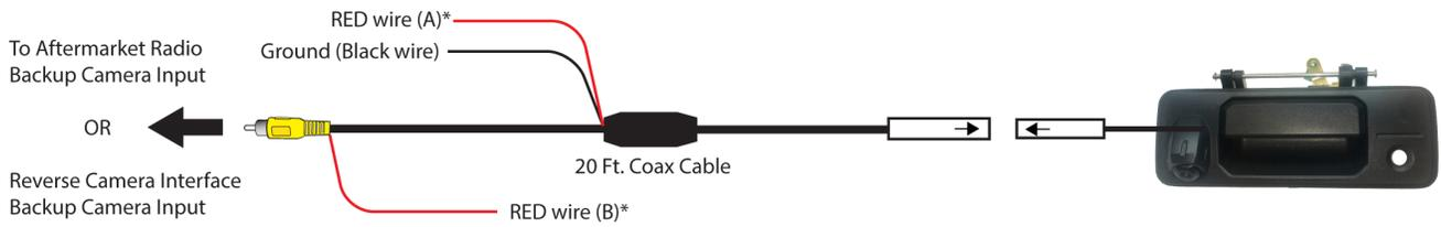
**\*NOTE:** The camera needs a +12V trigger. Power the camera at the headunit using RED Wire B or from the reverse light wire using RED Wire A. **DO NOT** connect both wires to +12V at the same time. Insulate the red wire that is not being used. Tap the Black wire to an existing ground lead, or ground Black wire securely to vehicle body metal.
