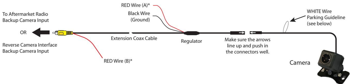
**\*NOTE:** The camera needs a +12V trigger. Power the camera at the headunit using RED Wire B or from the reverse light wire using RED Wire A. **DO NOT** connect both wires to +12V at the same time. Insulate the red wire that is not being used. Tap the Black wire to an existing ground lead, or ground Black wire securely to vehicle body metal.
