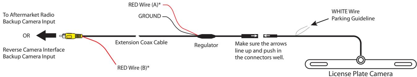
**\*NOTE:** To power the camera, use RED Wire A or B. If tapping power from the radio or RVC Interface, make sure to insulate RED Wire A to avoid it from shorting. If you will be tapping power from the reverse light +12V, insulate RED Wire B to avoid it from shorting. With either connection the Black GROUND wire needs to be connected to a solid chassis ground. For vehicles with manual transmission, we recommend tapping +12V power from the reverse light.
