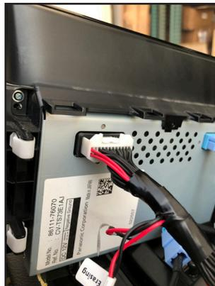
8. Plug the 24 pin power t-harness provided to the factory screen.
