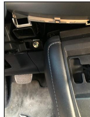
3. The left side trim is secured with a bolt under the ignition button.
