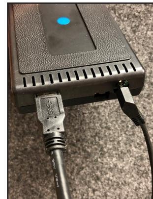
12. Plug in the extension USB cable and mic cable to the Smart-Play module.
