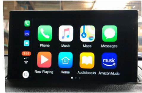
2. For a wired connection, plug in the smartphone's original charging/data cable to the USB port on the ACPMB-78Z harness. Image above shows the "Home Screen" for the Apple device once the smartphone is connected.
