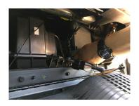
4. Plug the other 16-pin connector of the BTS-GM1X harness to the XM tuner.
