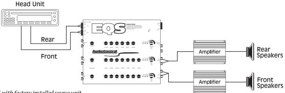
Figure 7: EQS with factory installed source unit
