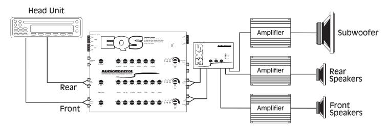
Figure 5: EQS with Four Channel Source Unit and 3XS crossover
