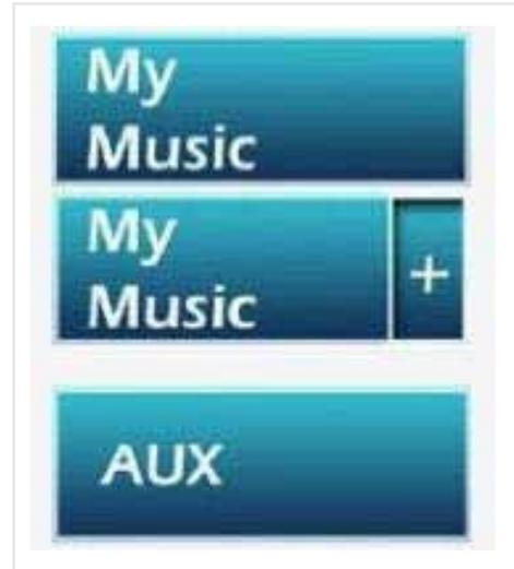
Step 2 -After activating the AUX audio source, Press and Hold the AUDIO/VIDEO button for 3 seconds to enter the interface module's input menu.
