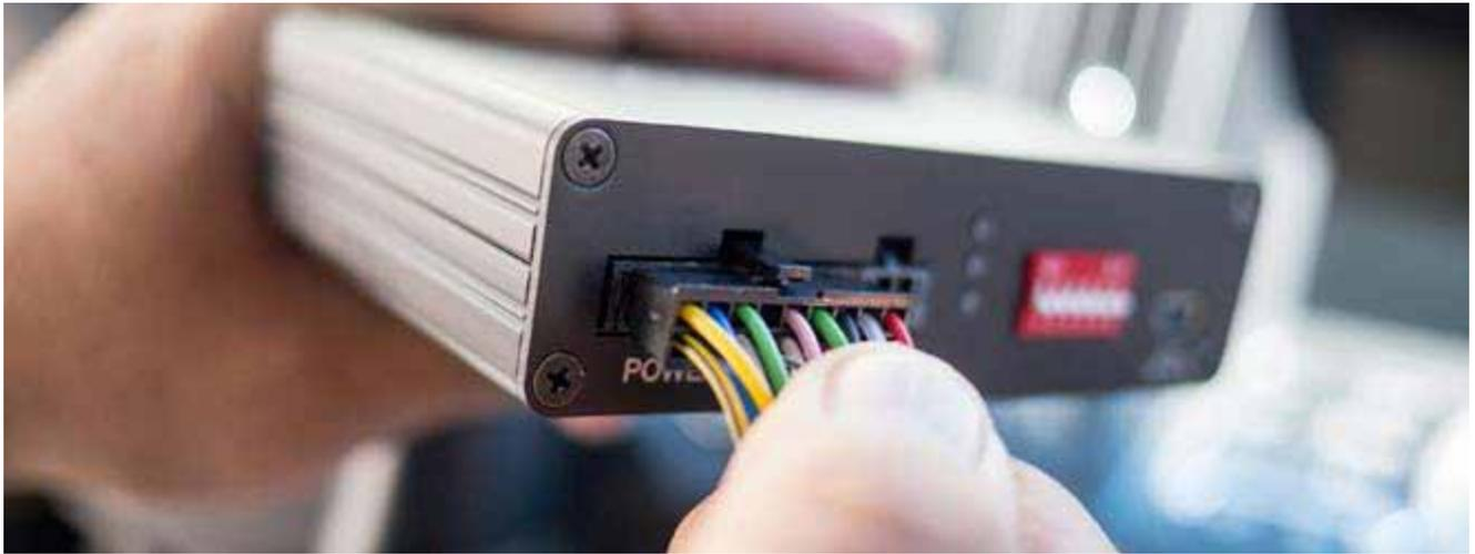
**Step 4** - After connecting the module, set the proper dip switches to the "ON" position. Make sure to set the AV sources being used to the "ON" position. **NOTE:** The Video In-Motion feature does not require activation. This feature is permanently ON and will not disturb the navigation GPS performance.
