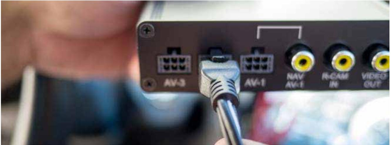
The Video Out port is to be used in vehicles that are equipped with Rear-Seat Entertainment Monitor or other external monitors. Included is a Video RCA Cable to be used with this feature. To retain the audio from the Rear-Seat Entertainment, use the attached Audio RCA's on the T-Harness.
