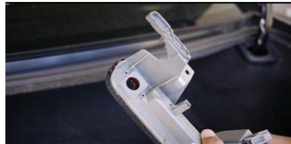
4. Insert the camera cable and the camera thru the hole but **DO NOT FULLY INSERT**. This will allow you to rotate the camera to the right position. Turn the ignition key to ON but do not start the engine. Put the gear in reverse and check the camera view. Adjust as necessary.
