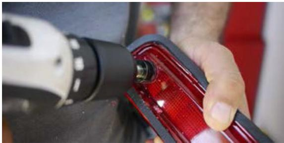
3. Turn over the third brake light assembly start drilling from the front side. Carefully drill thru the red plastic lens.
