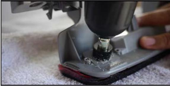
1. Remove the third brake light assembly. Use the supplied drill saw and drill a hole on the back side of the third brake light housing.
