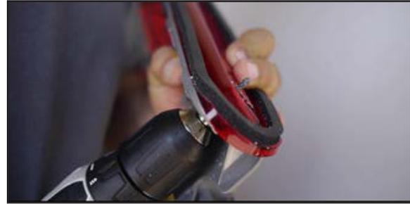
2. Continue drilling until the pilot drill bit is visible on the front side of the third brake light.
