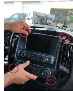
2. Carefully remove the radio trim with a plastic pry tool and pull outward.
