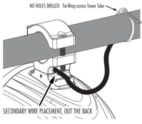
Step 9: Slide the wire jacket down thru the hole with grommet and wire. Snake the wire down to the bottom of the tower tube in a location that the wires can be attached to the audio (and lighting) system. Solder or butt connect the speaker wire coming from the tower to the speaker wire to the system. Then heat-shrink it for added protection from water/ moisture.
