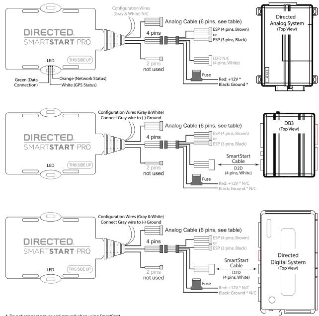
\* Do not connect power and ground when using SmartStart in a D2D configuration or damage may occur.
