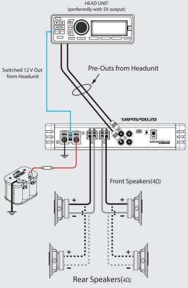
Total speaker impedance Total Speaker Impedance (MIN  $2\Omega$ )
