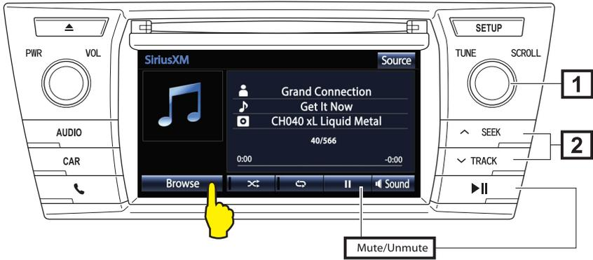
**1** Tuning Knob - switch to next available channel, depending on direction of rotation. (Tuning knob may not be available while radio is loading channel list.)
