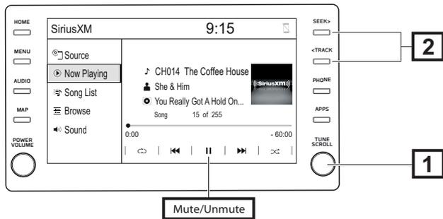
**1** Tuning Knob - switch to next available channel, depending on direction of rotation. (Tuning knob may not be available while radio is loading channel list.)
