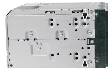
The metal side brackets will be attached to the sides of the Aftermarket Double DIN stereo.
